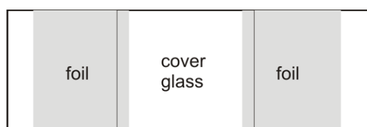
Figure 5: A sketch of a planar cell with parallel glass plates.
