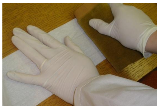
Figure 7: Rubbing the cover microscope glass by velvet in a certain direction
